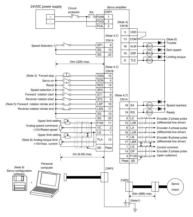
Note: 1. To prevent an electric shock, fit the supplied earth terminal (E) to the servo amplifier and always connect it to the earth (E) of the control box. (Refer to section 3.9.)
